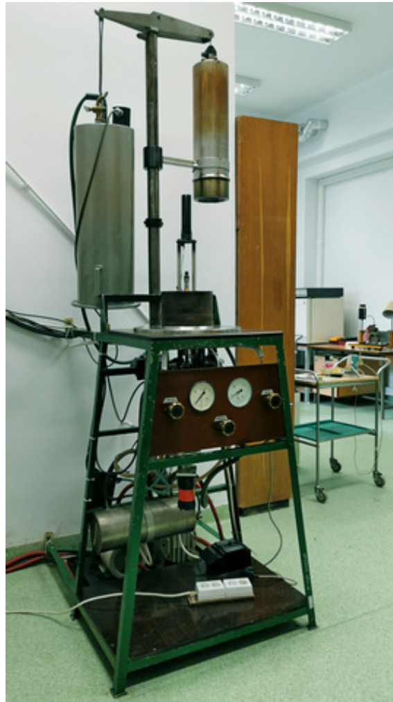
Fig. 4.11. Picture of the vertical Bridgeman equipment employed at Nicolaus Copernicus University in Toruń.
