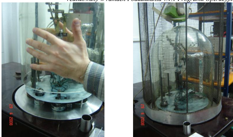
Fig. 10. Placing the bell jar (left) and metal net cover (right).
