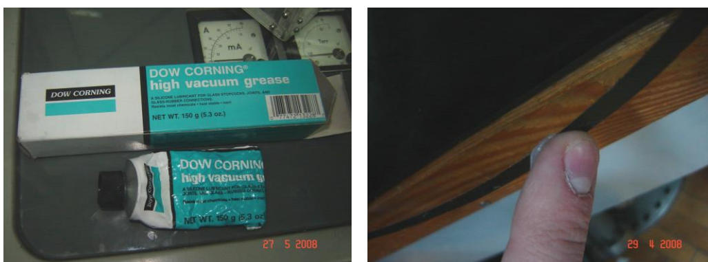
Fig. 9. The high vacuum grease (left), applying grease to the edges of bell jar (right).
