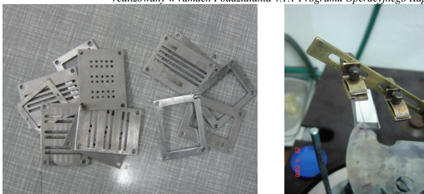
Fig. 7. The masks (left) for metal films and holder (right) for organic films in PVD system.
