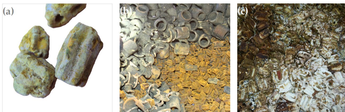
Figure 5. Images of used vanadium catalysts: (a) poisoning with arsenic compounds; (b) deactivation caused by dust agglomeration on the surface; (c) the effect of water vapour on the catalyst surface. http://www.sulphuric-acid.com/Sulphuric-Acid-on-the-Web/home.htm (28 April 2026; 13:30).
