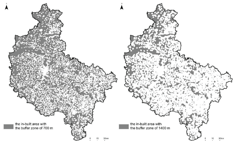
Figure 4. Area available for wind energy development—the built-up area with the buffer zones of 700 m and 1400 m in the Greater Poland Voivodeship (own calculations).
