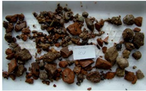
Fig. 6. Hydralit ZU – gravel fraction
