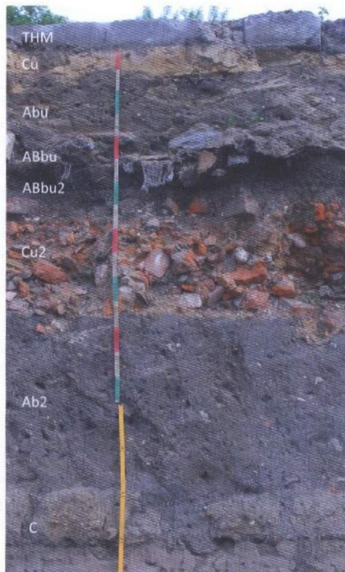
Fig. 4-3. Example of urban soil classified according to: WRB – Urbic Ekranic Technosol (Epiarenic, Calcaric, Endohyperartefactic, Skeletic). Soil Taxonomy: Artifactual, siliceous, mesic family of Anthropric Anthroportic Ustipsamments. KA 5 (soil form): Flat Syrozem from consolidated material above Colluvisol from dumped grit carbonate sand (Settlement construction waste) above tilted sand (Cover sand). Classification and Diagnostic System of Russian Soils: Lithostrat very intensive skeletal, loamy sandy, sealed by cobblestone cover.
