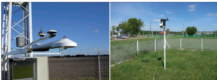
Fig. 4. A CNR4 net radiometer at the KON (left) and a Vantage Pro+ automatic weather station at the OME (photo by M. Kejna)
