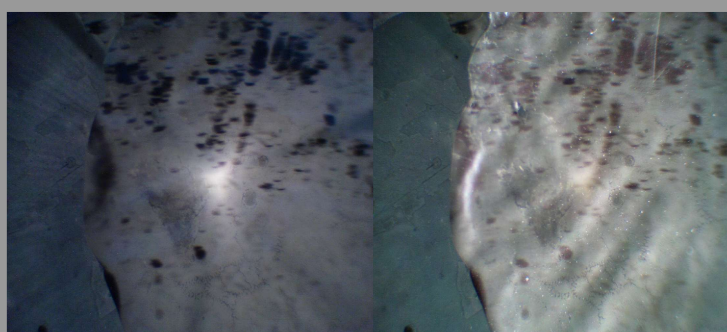
Photographic glass negative with silver-gelatin emulsion - dark field (left) and dark field + reflected side light (right)
