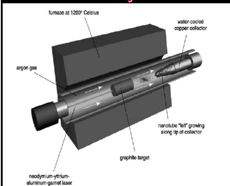
Fig. 5. Oven laser-vaporisation apparatus for the synthesis of single-walled carbon nanotubes [39].
